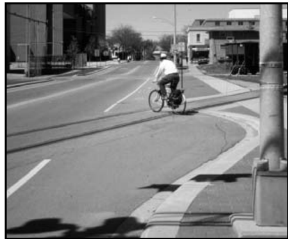
Sample Tapered Approach for Bicyclists to Cross the Railroad at a Safe Angle 15
